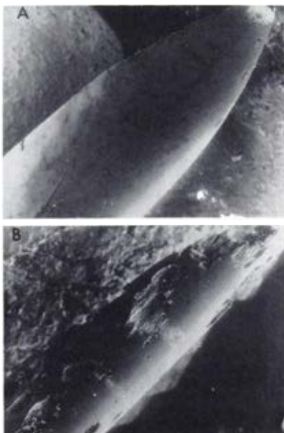
Fig. 4. A, normal appearance of tip of stainless steel electrode. Unused 18-gauge needle. \times 80 . B, corrosion damage to tip of stainless steel electrode. Needle after 1 mA for a total of 2 h. \times 80 .
